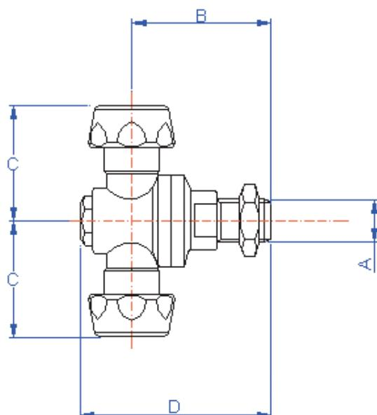
Nozzle complete with caps, nut and spray tips, with a maximum operating pressure of 40 bar; for use on air blast sprayers.
