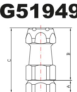
Nozzle complete with caps, nut and spray tips, with a maximum operating pressure of 40 bar; for use on air blast sprayers.
