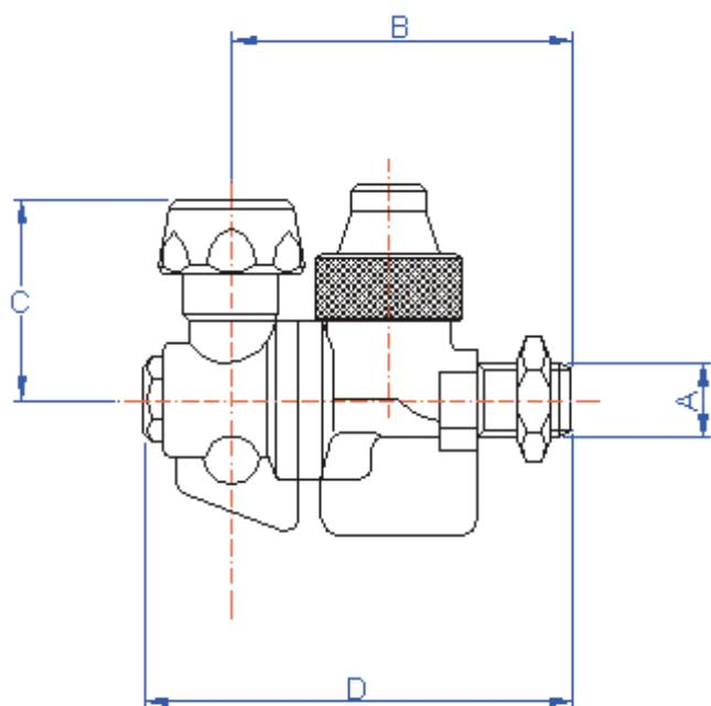
Nozzle complete with cap, nut and spray tip, with a maximum operating pressure of 40 bar; for use on air blast sprayers. The high quality materials, completely MADE IN ITALY, are Brass, Buna N, Viton, Ceramic plate and Stainless steel. "Open" and "Closed" positions obtained by turning the nozzle holder:
