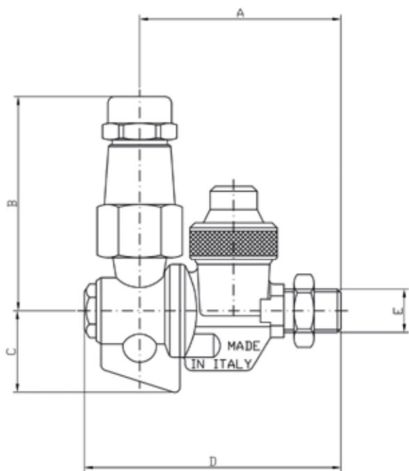
Nozzle complete with cap, nut and spray tip, with a maximum operating pressure of 40 bar, for use on air blast sprayers. The high quality materials, completely MADE IN ITALY, are Brass, Buna N, Viton, Ceramic plate and Stainless steel. "Open" and "Closed" positions obtained by turning the nozzle holder.
