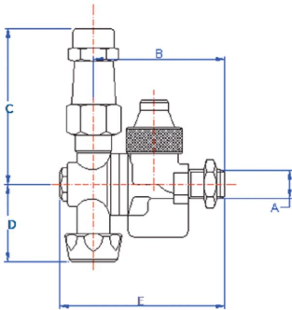
Nozzle complete with caps, nut and spray tips, with a maximum operating pressure of 40 bar, for use on air blast sprayers.
